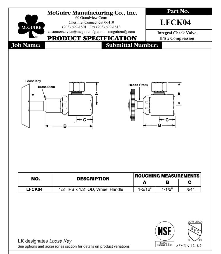
Chrome plated brass supply stop valve with spring actuated integral check valve and full turn brass stem. Inlet shall be (3/8, 1/2) inch (IPS, sweat, compression). Outlet shall be (3/8, 1/2) inch (IPS, compression). Integral check supply stop valve shall be McGuire \_\_\_\_\_\_. Integral check supply stop valve shall be certified or recognized by testing authority and bear manaufacturer and testing mark.
