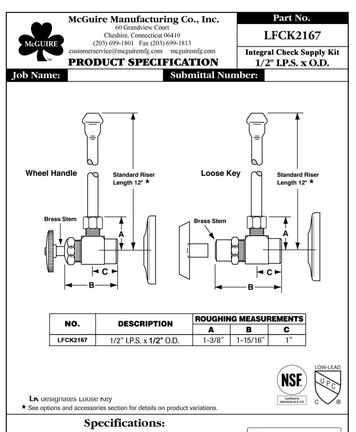
Supply kit shall include lead free integral check chrome plated brass stops with full turn brass stem, no plastic, (12, 15, 20) inch chrome plated copper risers and (shallow, deep, bell) (steel or brass) or (forged brass with set screw) flange. Inlet shall be (3/8, 1/2) inch (IPS, sweat, compression). Outlet shall be (3/8, 1/2) inch (IPS, compression). Supply kit shall be McGuire \_\_\_\_\_\_. Supply kit shall be certified by recognized authority and bear manufacturer and testing mark.
