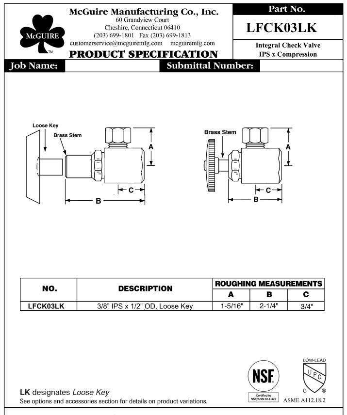
Chrome plated brass supply stop valve with spring actuated integral check valve and full turn brass stem. Inlet shall be (3/8, 1/2) inch (IPS, sweat, compression). Outlet shall be (3/8, 1/2) inch (IPS, compression). Integral check supply stop valve shall be McGuire \_\_\_\_\_\_. Integral check supply stop valve shall be certified or recognized by testing authority and bear manaufacturer and testing mark.
