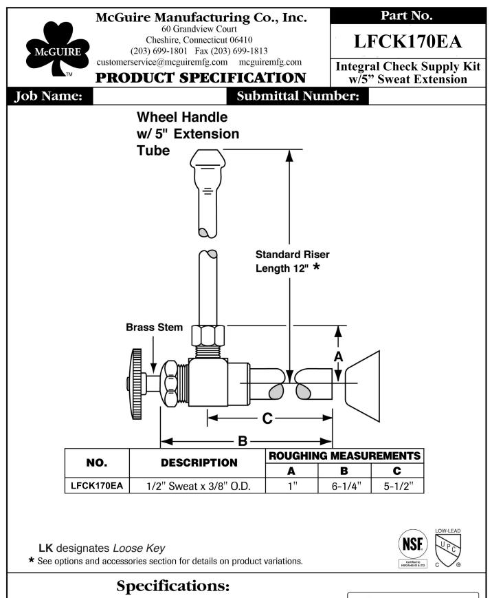
Supply kit shall include lead free chrome plated brass integral check supply stop valves with full turn brass stem, no plastic, (12, 15, 20) inch chrome plated risers and (shallow, deep, bell) (steel, brass) or (forged brass with set screw) flange. Inlet shall be 1/2 inch (IPS, sweat, compression). Outlet shall be 3/8 inch (IPS, compression). Supply kit shall be McGuire \_\_\_\_\_\_. Supply shall be certified by recognized authority and bear manufacturer and testing mark.
