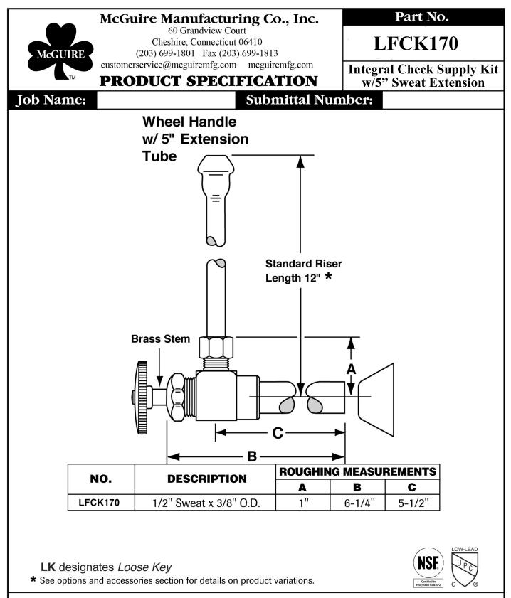
Supply kit shall include lead free chrome plated brass integral check supply stop valves with full turn brass stem, no plastic, (12, 15, 20) inch chrome plated risers and (shallow, deep, bell) (steel, brass) or (forged brass with set screw) flange. Inlet shall be 1/2 inch (IPS, sweat, compression). Outlet shall be 3/8 inch (IPS, compression). Supply kit shall be McGuire \_\_\_\_\_\_. Supply shall be certified by recognized authority and bear manufacturer and testing mark.
