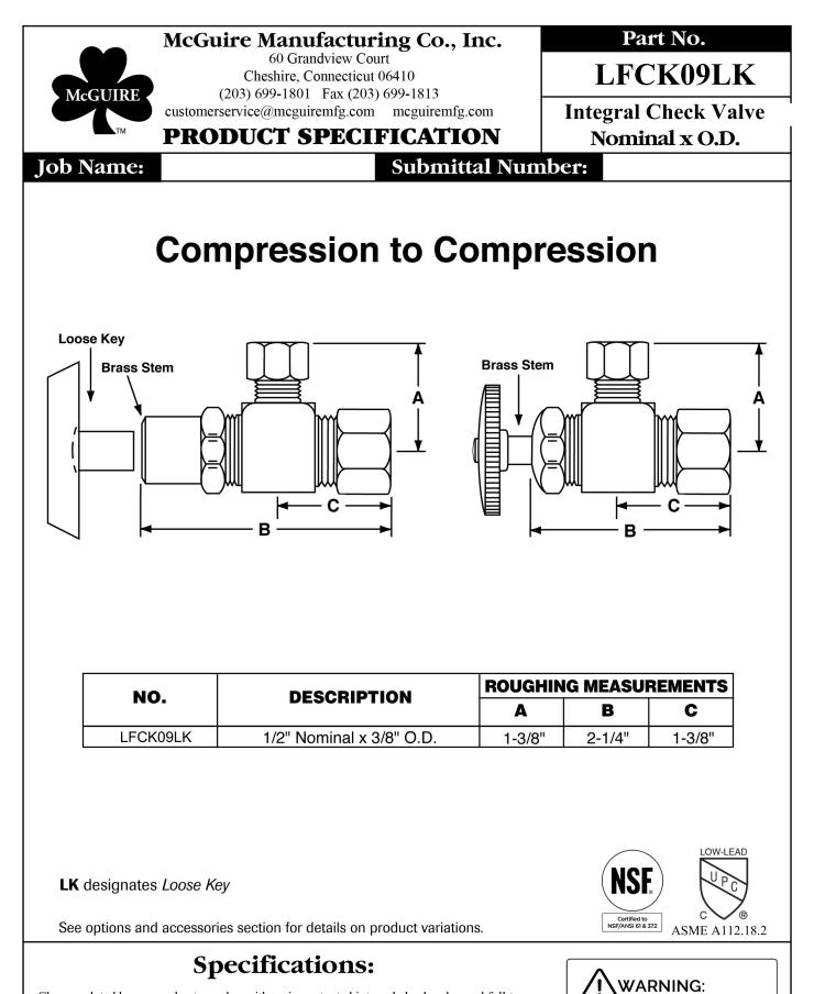
Chrome plated brass supply stop valve with spring actuated integral check valve and full turn brass stem. Inlet shall be (3/8, 1/2) inch (IPS, sweat, compression). Outlet shall be (3/8, 1/2) inch (IPS, compression). Integral check supply stop valve shall be McGuire
