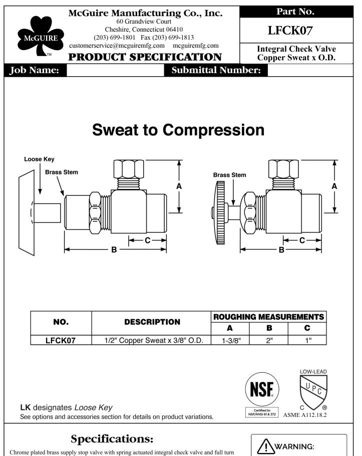
brass stem. Inlet shall be (3/8, 1/2) inch (IPS, sweat, compression). Outlet shall be (3/8, 1/2) inch (IPS, compression). Integral check supply stop valve shall be McGuire \_\_\_\_\_\_.
