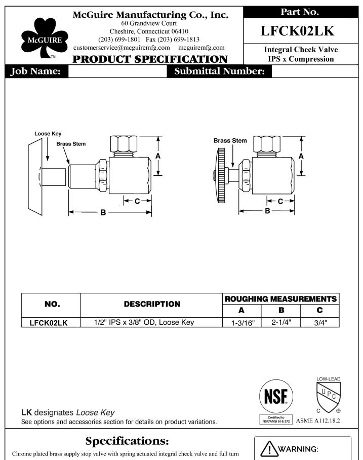
brass stem. Inlet shall be (3/8, 1/2) inch (IPS, sweat, compression). Outlet shall be (3/8, 1/2) inch
